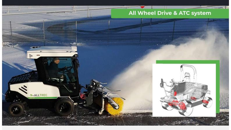
**Advanced Torque Control**, specially developed for the 8015F. This system ensures maximum grip and good maneuverability, but above all great handling and power delivery in the different conditions that users encounter during work.
